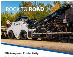
Designed with safety and operator comfort in mind, the Shuttle Buggy® SB-3000 material transfer vehicle features adaptive cruise control, bright LED lighting and fourwheel steering.
