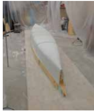
Figure 6: Finished Mold Ready for Pour
