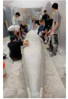
Figure 11: Finishing Concrete Placement
