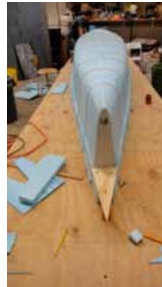
Figure 3: Hot Wire Cutting Complete
