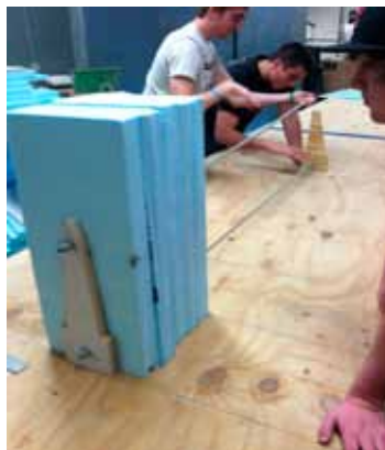
Figure 2: Bolting together Cross-Sections for Cutting
