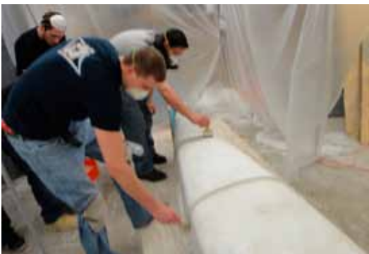
Figure 5: Applying Form Release to the Mold
